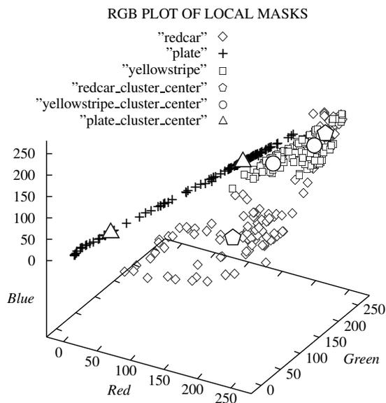
Figure 2: Pixels of the three masks highlighted in figure 1 a.) together with the two cluster centers of each mask.
