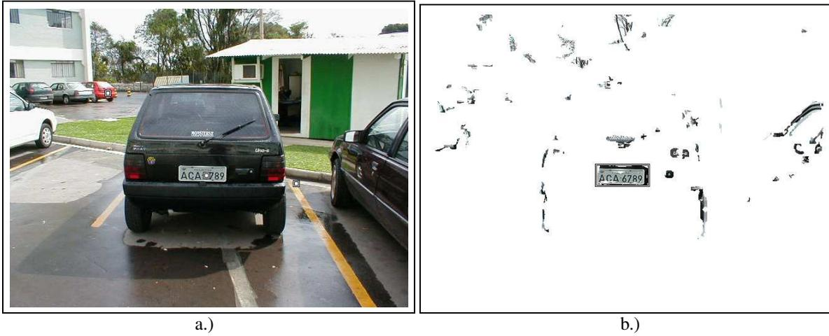
Figure 1: Example result. a.) Original image with three  $11 \times 11$  masks used for the determination of the two color modes. First mask "redcar" from rear part of small red car (right car of the three car group). Second mask "yellowstripe" from area of parking lot on the right side of the central vehicle. Third mask "plate" from transition area of license plate of the same car; b.) bounding boxes of plate candidates.
