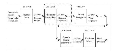
Fig. 1. Multilevel multi-decision Dictation/Translation Machine structure
